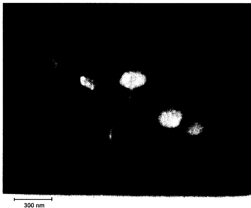
FIGURE 2 Electron micrograph of 3-sn-phosphatidylcholine (egg yolk) liposomes obtained after extrusion through a 400 nm pore polycarbonate membrane
